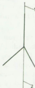
Fig. 2. The position of the centre of gravity. 1—a flexible thread; 2—the plane of the axes.
