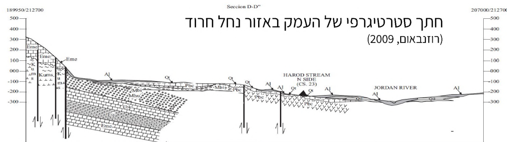
Figure 7. Cross section cutting the Harod Valley and the Harod River, east of Mount Barkan to the Jordan River, crossing the northern part of the northern body of the Bet She'an tufa. E
